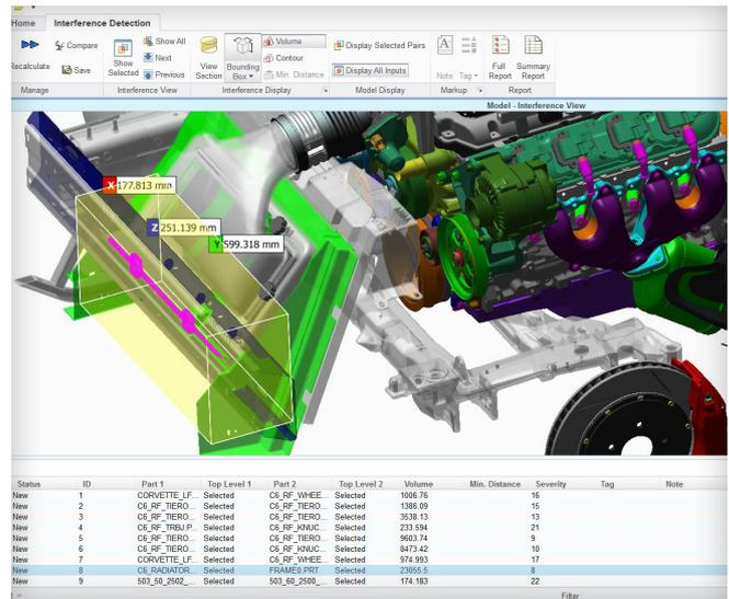
Detect and analyze clash issues with the optional Creo View Interference Analysis module.
